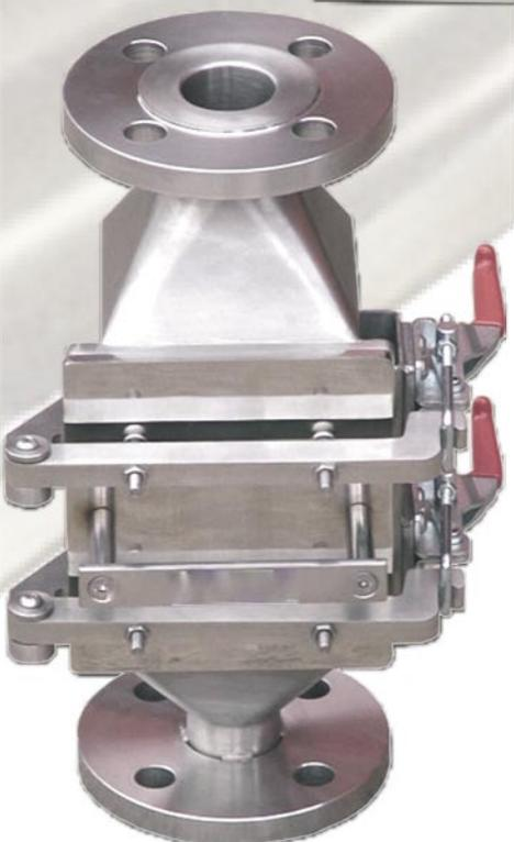
**AGHD and APG grid magnet units** for high pressures and usage in pneumatic lines (compound, liquids etc) for normal or high temperatures. Construction only with flange connection or pipe connection. With end switch if desired. Easiest cleaning, food save construction (100% stainless steel 1.4301 electropolished)
