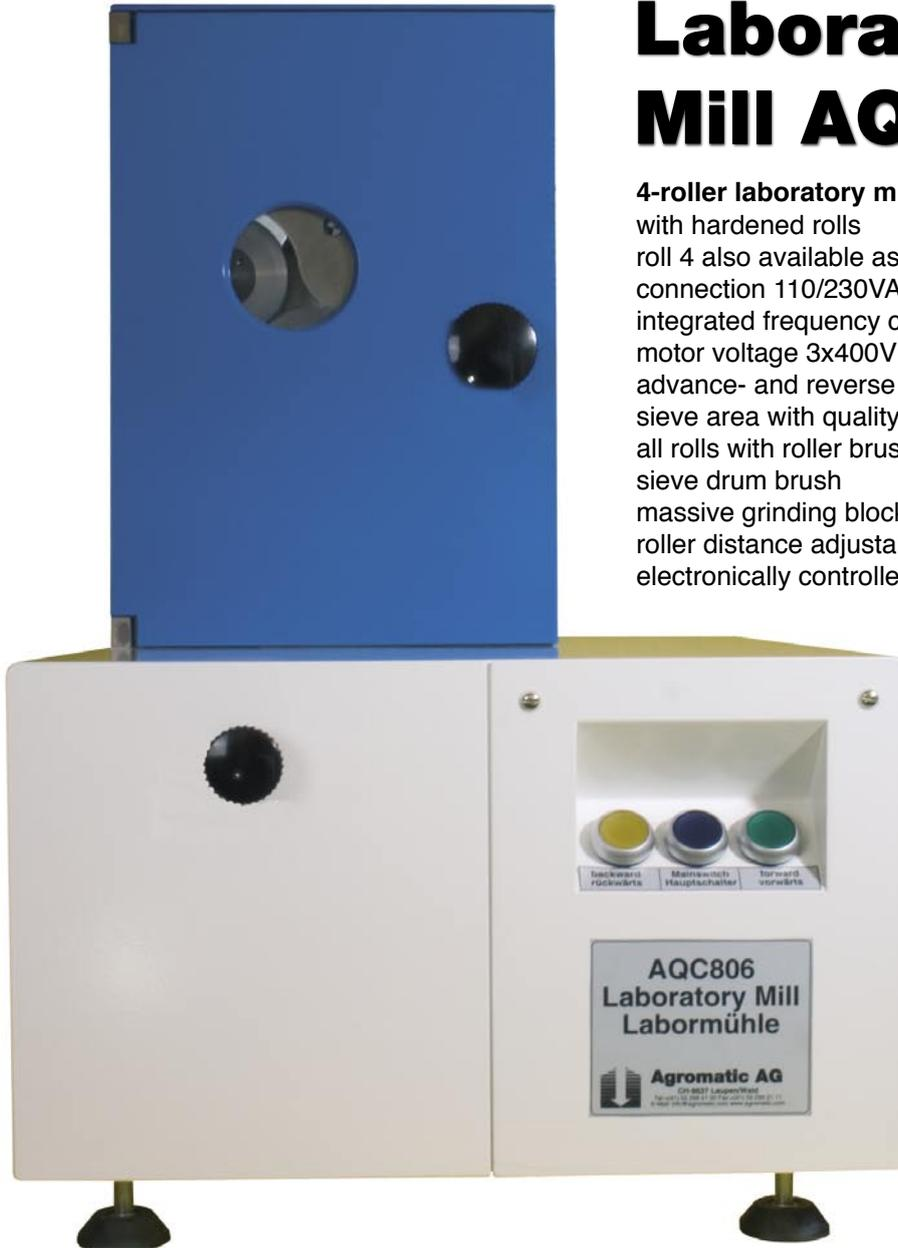
For production of flour from grain samples for further tests and analysis.
